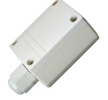
The sensor measures the temperature by use of a NTC, PT, or NI-sensing element. The sensing element is either a glass packed thermistor with a negative temperature coefficient, a platinum film or a nickel thin layer based probe. Its resistance changes according to the temperature. The change follows a specified curve. Contact our sales department for curves not yet listed below.
