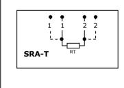
Platinum film and N11000 sensors use double contacts in order to compensate conductor resistance.
