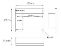
If using HDA0002 DIN rail adapter brackets the overall depth from the gear plate to the front surface of the device is 45.5 mm
